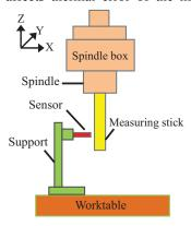
**Fig. (3).** Measurement of X-axis thermal errors.
