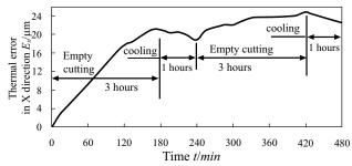
Fig. (4). Thermal errors in X-axis direction.
