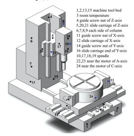
Fig. (1). Main thermal sources of a CNC machine tool.
