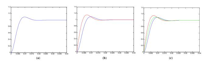
Fig. (4). System response with different zeros.
