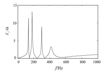
Fig. (12). Impedance-frequency characteristics of PPF.
