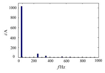
Fig. (5). Frequency spectrum of the current which TCR injecting into phase C under symmetrical voltage.
