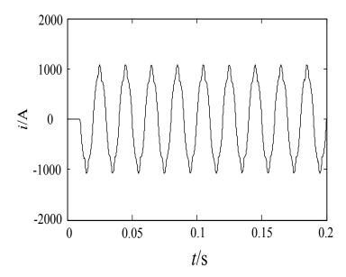
Fig. (6). Waveform of current which TCR injecting into phase C under asymmetrical voltage.
