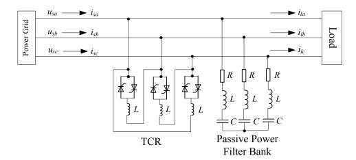
Fig. (1). Topology of TCR compensation system.
