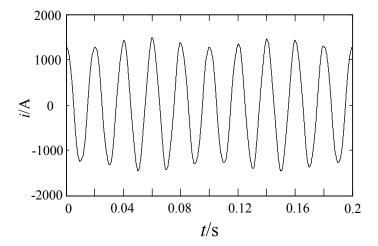
Fig. (10). Current waveform of power system after PPF operating.
