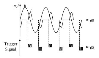
Fig. (2). Waveform of power system voltage and TCR current.
