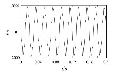
Fig. (8). Current waveform of power system before PPF operating.
