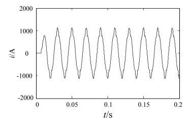
Fig. (4). Waveform of the current which TCR injecting into phase c under symmetrical voltage.
