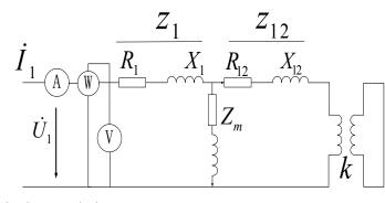
Fig. (1). Wiring diagram of short circuit test method.
