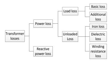
Fig. (2). Composition transformer losses.
