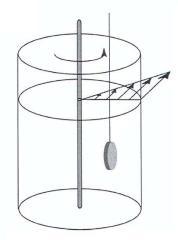
Fig. (1). Illustration of rotating beaker with a tablet fixed on a steel wire. The beaker is glued to the centrally placed rod at the bottom so that when the rod is rotated at fixed rpm the beaker also rotates at the same rpm (reproduced with permission from ref [46]).
