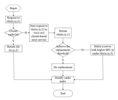
Fig. (3). Replacement flow and collaboration in a Heterogeneous DCCS.
