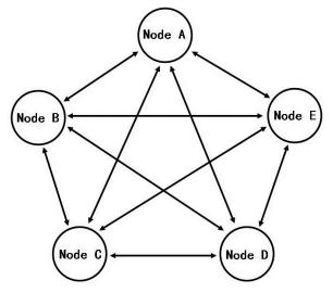
Fig. (8). Example of the Mesh Topology.
