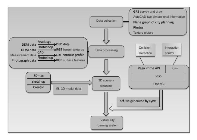
Fig. (2). The procedure of the roaming system of virtual city.
