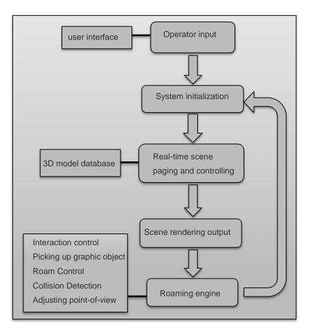
Fig. (1). Engine structure frame of the roaming system of virtual city.
