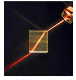
**Fig. (1).** A view of a light beam propagating in water showing the sharp angle of refraction at the water surface, and the preservation within water of the refracted beam with only partial dispersion.
